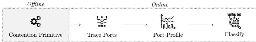
Fig. 2: PortPrint has four stages: (1) Creating port-contention primitives in the offline phase either dynamically or based on reverse-engineered information, (2) tracing the execution ports during victim execution, (3) converting the traces to a port-contention profile, and (4) classifying the profiles.
