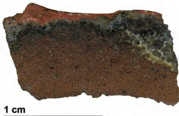
Figure 1: Section of open-faced crucible Fd. Nr. 410 with red glassy slag on the interior associated with dark vitrification of the ceramic. The ceramic is thoroughly burned and has a homogeneous texture (Keyence digital microscope image).
