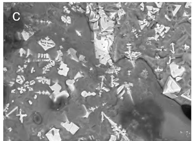
Figure 4: Crucible Fd. Nr. 3342 SEM-backscatter images. a) Section showing the frothy vitrified repair layer and the denser crucible ceramic. The white areas are silver corrosion products and metallic silver in the crucible ceramic pores. b) Mounted and polished section showing the repair layer and the crucible ceramic. c) Magnetite crystals in the glass on the crucible exterior. No scale.
