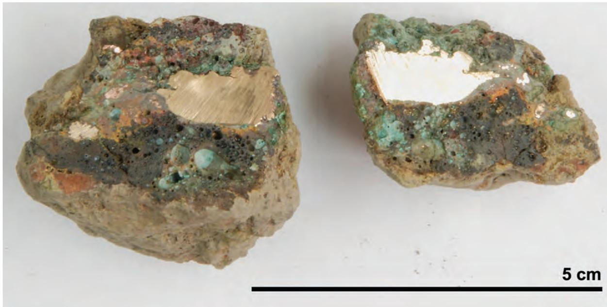
Figure 5: Section of hearth fragment Fd. Nr. 1032. The section reveals bronze casting waste and copper prills and frothy vitrified ceramic and glassy slag.
