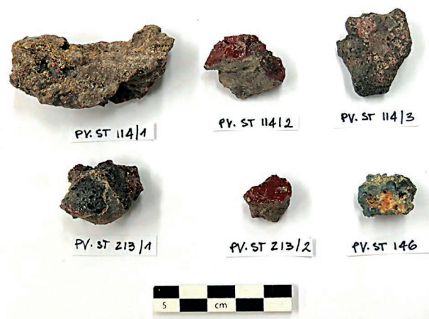
Figure 2. Example of the diversity of the metallurgical debris recovered at San Tommaso (Pavia). The investigation of the materials was performed using optical microscopy, X-Ray fluorescence, and scanning electron microscopy.
