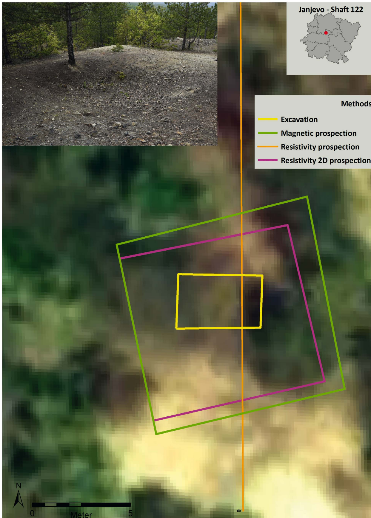
Figure 15. Janjevo, shaft 122, overview of all methods: magnetic and resistivity (2D) prospection and excavation. The photo shows the mining depression and the ring-shaped dump of shaft 122 before the excavation. Illustration: B. Sikorski; photo: archive DBM, G. Körlin.
